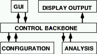
Tcl programmers are familiar with using Tcl as the backbone, with compiled extensions like Tk or BLT for the GUI and output, and compiled extensions or standalone applications for the analysis subsystem. This "Tcl as backbone" architecture provides a quick and flexible framework for developing applications.
